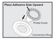
Installing the probe cover before measurement
